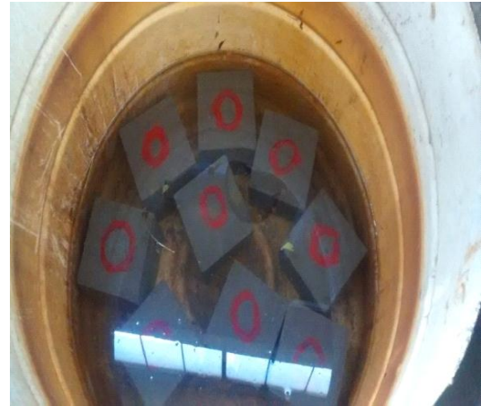
Fig 2 Immersing of cubes in water until tested
