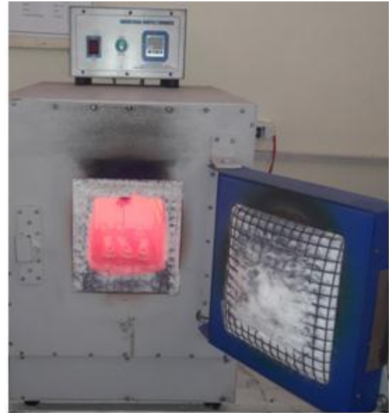
Figure 4 High Temperature Corrosion in Industrial Muffle Furnace
