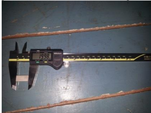
Figure3: Vernier caliper with least count 0.02
