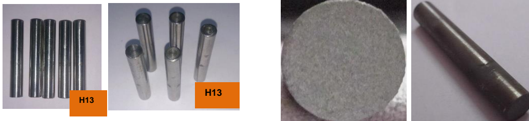
Fig. 1 Camera macrographs of steel pins Fig. 2 the camera macrographs of as-sprayed coatings on H13 substrate (a) top surface (b) full sample
