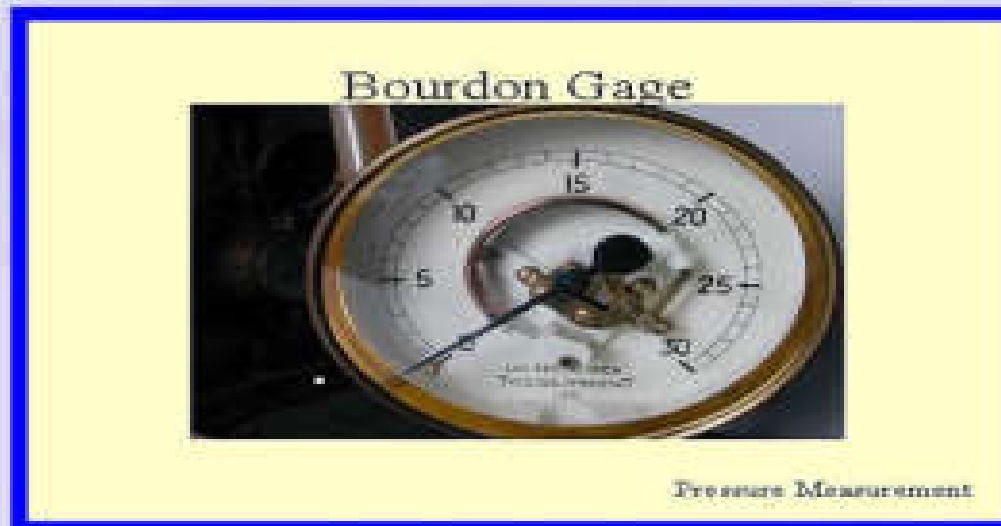
Figure 69 Photograph of a Bourdon gage taken from the web (Dr. Pravin Vama, Mount Allison University, Sackville, New Brunswick Canada )
