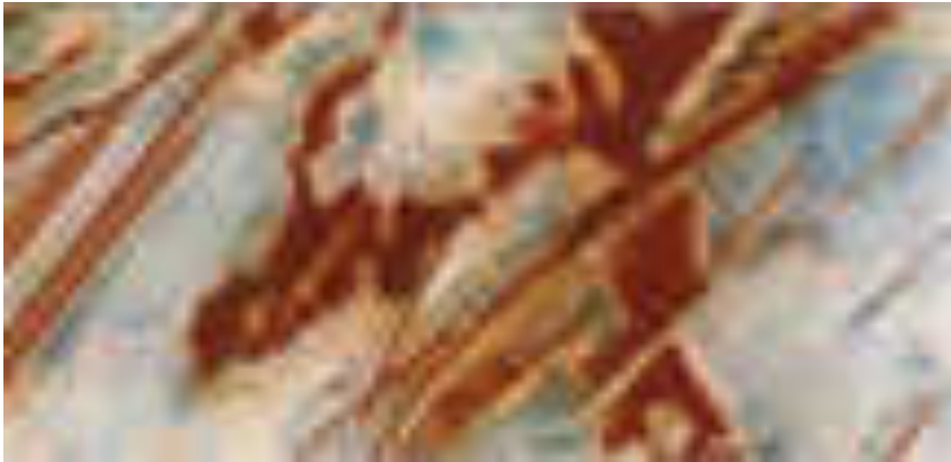
Fig. 13: High magnification view (400x) of the white cast iron specimen shown in Fig. 11, etched with alkaline sodium picrate. After Mrs. Janina Radzikowska, Foundry Research Institute in Kraków, Poland
