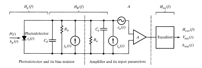
The binary digital pulse train incident on the photodetector can be written in the following form:
