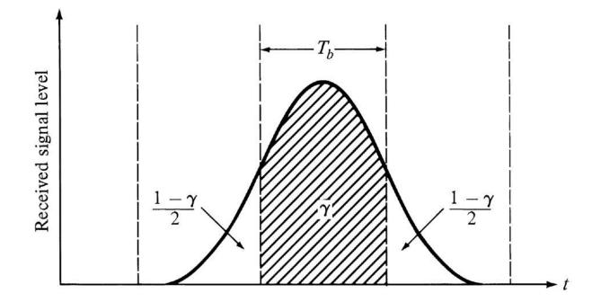
Pulse spreading in an optical signal, after traversing along optical fiber, leads to ISI. Some fraction of energy remaining in appropriate time slot is designated by  $\mathcal{V}$ , so the rest is the fraction of energy that has spread Into adjacent time slots.
