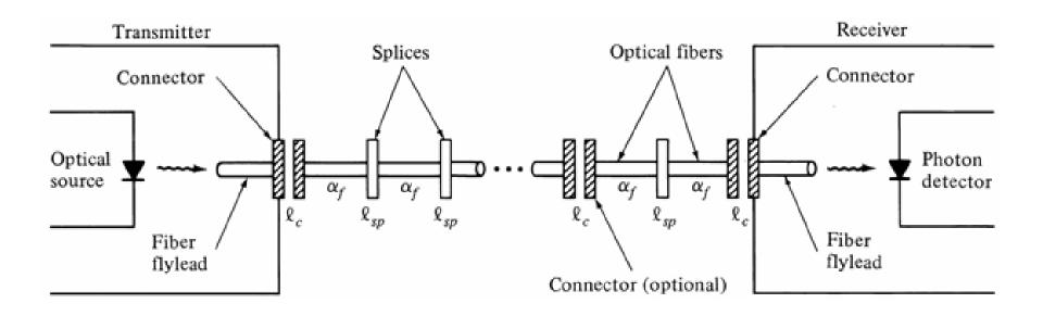
$P_{T}[dB] = P_{s}[dBm] - P_{R}[dBm] \text{ Total Power Loss}$  $P_{T} = 2l_{c}[dB] + \alpha_{f}[dB / km] \times L[km] + \text{System Margin}$
