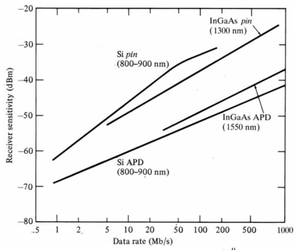
The Si PIN & APD and InGaAsP PIN plots for BER= $10^{-9}$ . The InGaAs APD plot is for BER= $10^{-11}$ .
