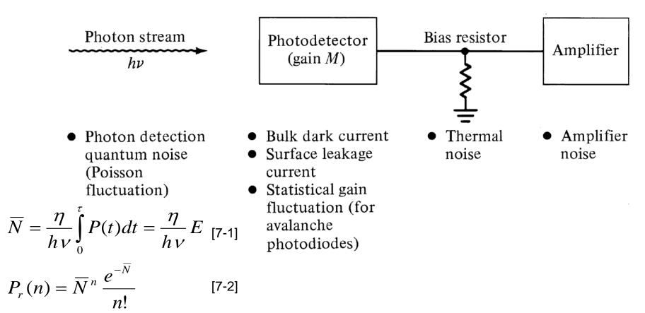
$\overline{N}$  is the average number of electron-hole pairs in photodetector,
