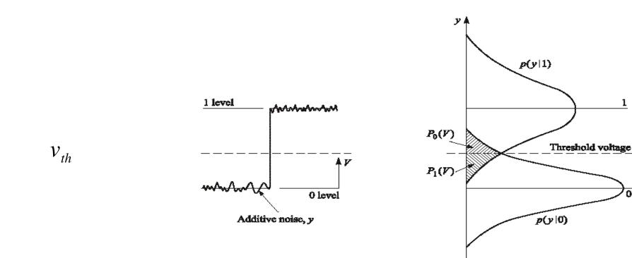
Probability distributions for received logical 0 and 1 signal pulses. the different widths of the two distributions are caused by various signal distortion effects.
