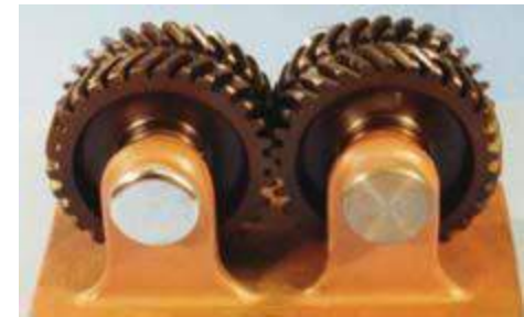
Herringbone gears (or double-helical gears)
