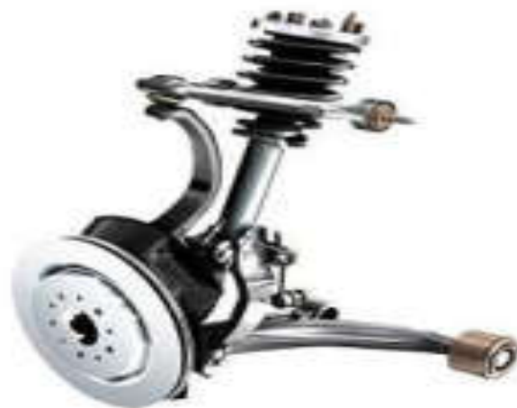
The shock absorber usually consists of two parts: a spring and a damper or dashpot .
