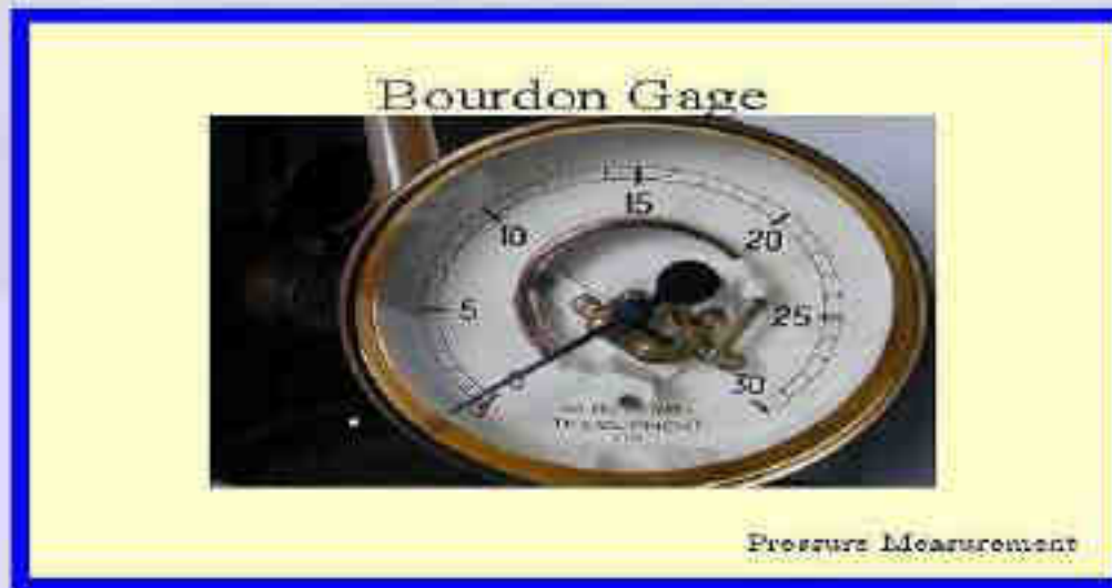
Figure 69 Photograph of a Bourdon gage taken from the web (Dr. Pravin Varma, Mount Allison University , Sackville, New Brunswick Canada)
