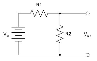
$V_{out} = I_{R1} R_2$ . KVL says the voltage around the loop including the battery and both resistors is 0, therefore  $V_{in} = V_{R1} + V_{out}$ , or  $V_{in} = I_{R1} R_1 + I_{R1} R_2$ . Thus,  $I_{R1} = V_{in} / (R_1 + R_2)$ , and
