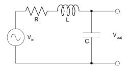
Derive the filter gain of the pictured circuit. Plot the magnitude and phase of the filter for L = 6.3e-6 [H], R = 16 [ $\Omega$ ], and C = 1.0e-7 [F]. For extra credit, also plot for R = 7 [ $\Omega$ ] and 50 [ $\Omega$ ].
