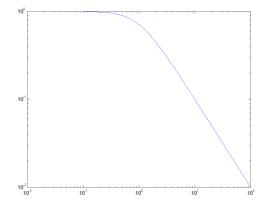
Magnitude and phase plots of A, where RC=1. The magnitude plot is log/log, while the phase plot is linear radians vs. log freq.
