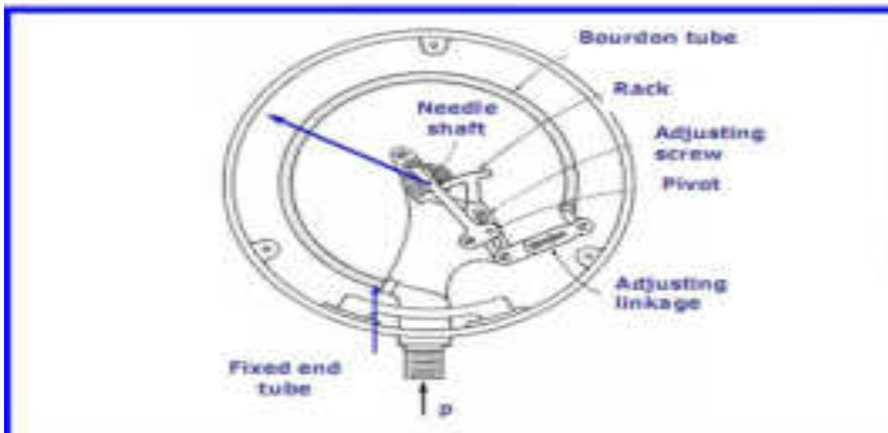
**Figure 68 Schematic of a Bourdon pressure gage**
