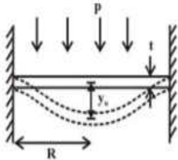
Fig. 2 Displacement of a diaphragm
